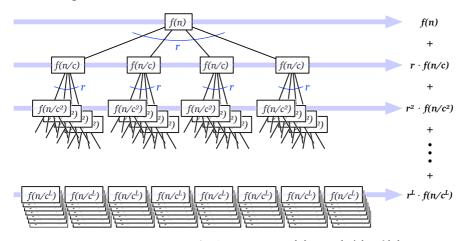
**Figure 1.9.** A recursion tree for the recurrence T(n) = r T(n/c) + f(n)
