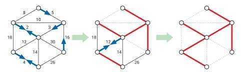
**Figure 7.3.** Borůvka's algorithm run on the example graph. Thick red edges are in *F*; dashed edges are useless. Arrows point along each component's safe edge. The algorithm ends after just two iterations.
