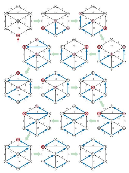
**Figure 8.15.** A complete run of Dijkstra's algorithm on a graph with negative edges. At each iteration, bold edges indicate predecessors; shaded vertices are in the priority queue; and the bold vertex is the next to be scanned. Compare with Figure 8.17.
