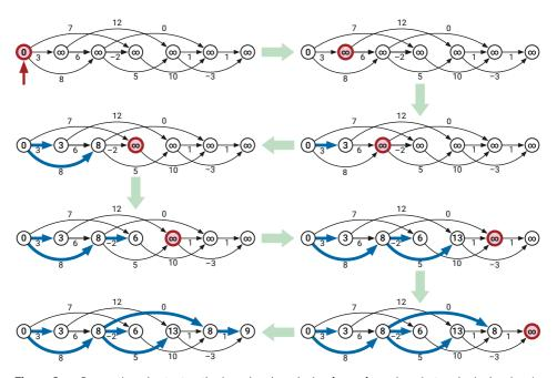
**Figure 8.9.** Computing shortest paths in a dag, by relaxing **incoming** edges in topological order. In each iteration, bold edges indicate predecessors, and the bold vertex is about to be scanned. Compare with Figure 8.10.
