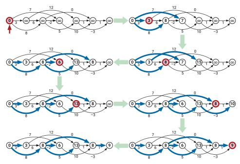
**Figure 8.10.** Computing shortest paths in a dag, by relaxing **outgoing** edges in topological order. In each iteration, bold edges indicate predecessors, and the bold vertex is about to be scanned. Compare with Figure 8.9.
