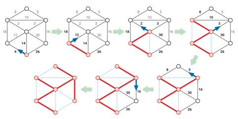
**Figure 7.4.** Jarník's algorithm run on the example graph, starting with the bottom vertex. At each stage, thick red edges are in *T*, an arrow points along *T*'s safe edge; and dashed edges are useless.
