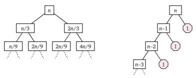
Figure 1.11. Recursion trees for quicksort with good pivots (left) and with worst-case pivots (right)
