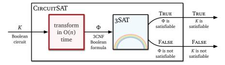
Figure 12.6. A polynomial-time reduction from CIRCUITSAT to 3SAT.
