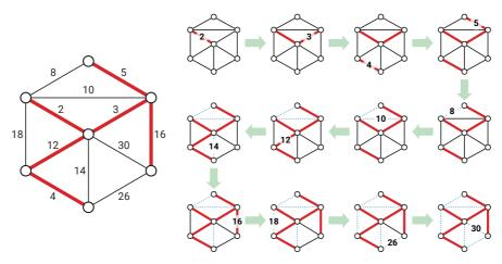
**Figure 7.6.** Kruskal's algorithm run on the example graph. Thick red edges are in F; thin dashed edges are useless.
