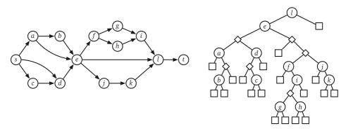
**Figure 10.13.** A series-parallel graph and a corresponding decomposition tree. Squares in the decomposition tree are leaves; diamonds are parallel nodes.
