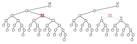
Figure 1.27. Deleting a central vertex in a 34-node binary tree, leaving subtrees with 14, 7, and 12 nodes.
