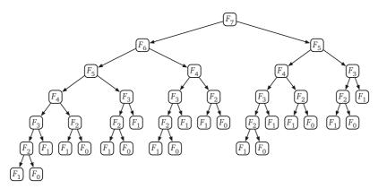
**Figure 3.1.** The recursion tree for computing  $F_7$ ; arrows represent recursive calls.
