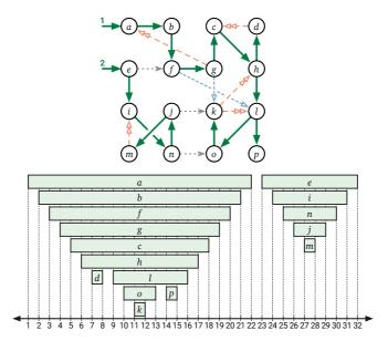
**Figure 6.4.** A depth-first forest of a directed graph, and the corresponding active intervals of its vertices, defining the preordering *abfachlokpeinim* and the postordering *dkoplhcgfbaminie*. Forest edges are solid; dashed edges are explained in Figure 6.5.
