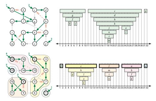
**Figure 6.17.** The Kosaraju-Sharir algorithm in action. Top: Depth-first traversal of the reversed graph. Bottom: Depth-first traversal of the original graph, visiting root vertices in reversed postorder from the first traversal.
