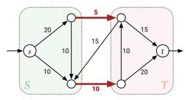
**Figure 10.3.** An (s, t)-cut with capacity 15. Each edge is labeled with its capacity.
