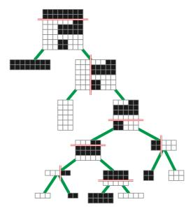
Figure 3.7. A guillotine subdivision with size 8 and depth 5.
