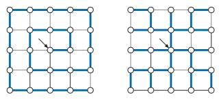
Figure 5.12. A depth-first spanning tree and a breadth-first spanning tree of the same graph, both starting at the center vertex.
