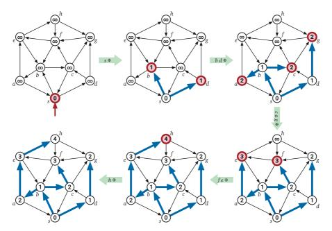
**Figure 8.6.** A complete run of breadth-first search in a directed graph. Vertices are pulled from the queue in the order  $s \not = b d \not = c a g \not = f e \not = h \not = f$ , where  $\not = f$  is the end-of-phase token. Bold vertices are in the queue at the end of each phase. Bold edges describe the evolving shortest path tree.
