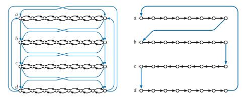
**Figure 12.19.** Left: Variable gadgets and connectors in G, for any formula with 4 variables and 4 clauses. Right: The Hamiltonian cycle in G corresponding to the assignment a = b = d = True and c = False
