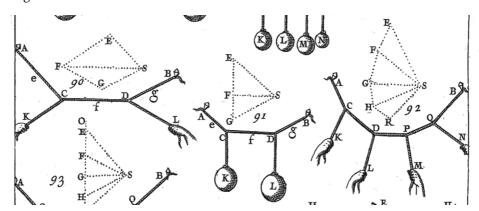
**Figure 5.3.** Reciprocal force diagrams (dotted), from Varignon's posthumous *Nouvelle mécanique*, *ou statique*, *dont le projet fut donné en MDCLXXXVII* [New mechanics, or statics, whose project was given in 1687] (See Image Credits at the end of the book.)
