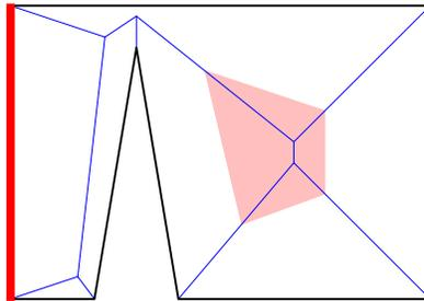
**Figure 6.** The roof of a weighted polygon is not the lower envelope of its slabs. The leftmost edge has higher weight than the other edges, and its edge slab cuts through the roof in the shaded region.
