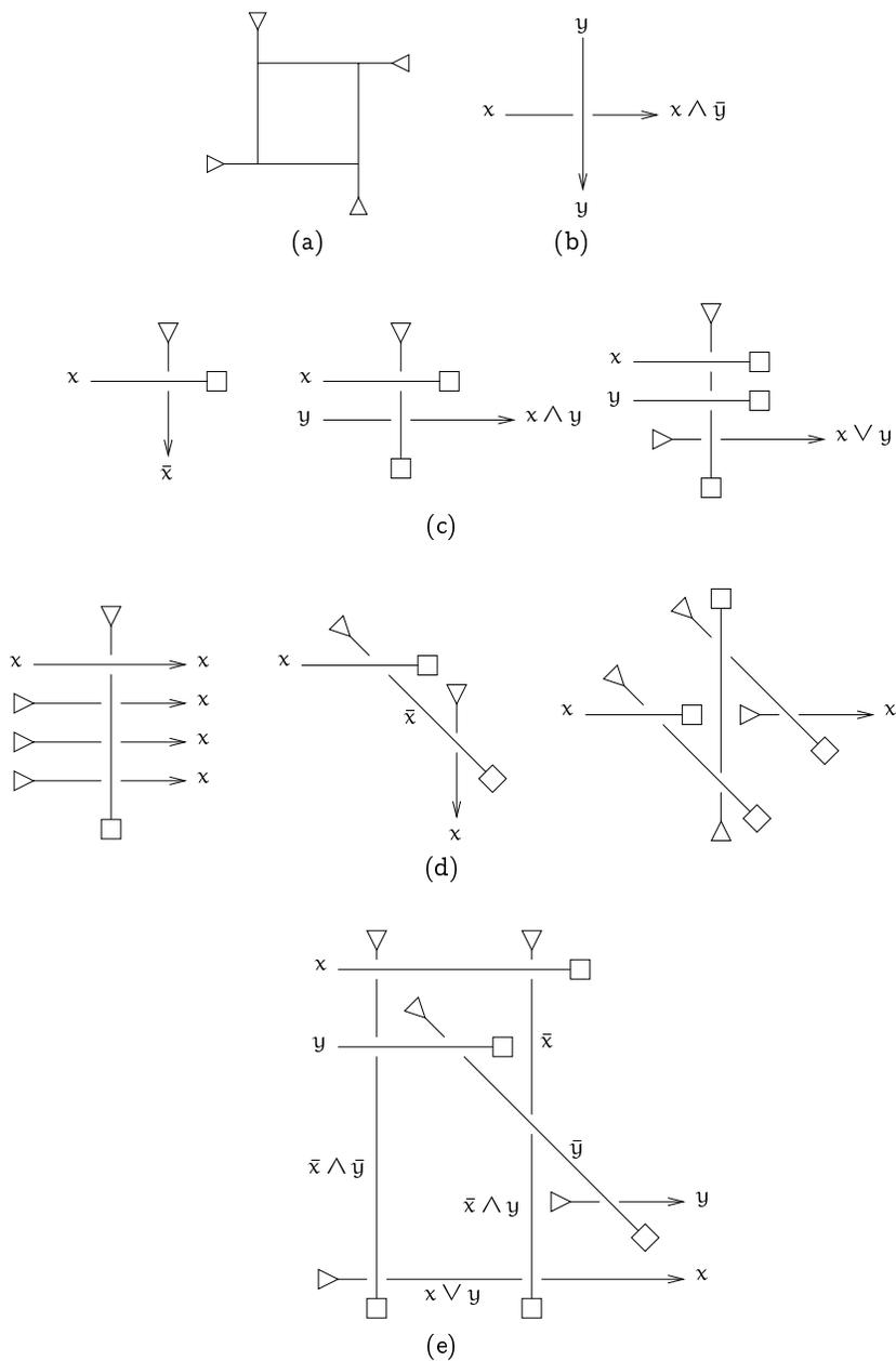
**Figure 8.** Reducing a boolean circuit to a motorcycle graph. Triangles denote the starting positions and directions of motorcycles. (a) A stopper, hereafter drawn as a square. (b) The effect of a potential collision. (c) NOT, AND, and OR gates. (d) Fanout, bend, and delay gadgets built out of inverters. (e) A crossover gadget.
