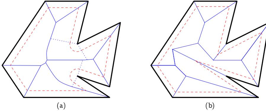
**Figure 1.** Skeletons and offset curves of a simple polygon. (a) The medial axis (solid), the Voronoi diagram (solid and dotted), and a rounded offset curve. (b) The straight skeleton and a mitered offset polygon.
