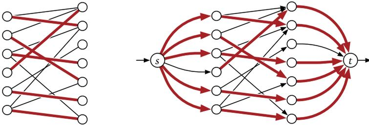
**Figure 11.2.** A maximum matching in a bipartite graph  $G$ , and the corresponding maximum flow in  $G'$ .
