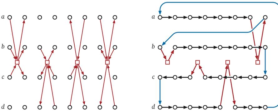
**Figure 12.20.** Left: Clause gadgets for the formula  $(a \vee b \vee c) \wedge (b \vee \bar{c} \vee \bar{d}) \wedge (\bar{a} \vee c \vee d) \wedge (a \vee \bar{b} \vee \bar{d})$ . Right: A Hamiltonian cycle in  $H$  corresponding to the satisfying assignment  $a = b = d = \text{TRUE}$  and  $c = \text{FALSE}$ .
