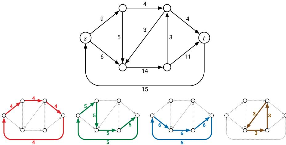
Figure 10.9. Decomposing a circulation into weighted directed cycles.
