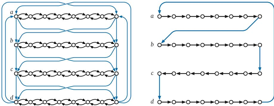
**Figure 12.19.** Left: Variable gadgets and connectors in  $G$ , for any formula with 4 variables and 4 clauses. Right: The Hamiltonian cycle in  $G$  corresponding to the assignment  $a = b = d = \text{TRUE}$  and  $c = \text{FALSE}$
