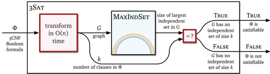
Figure 12.7. A polynomial-time reduction from 3SAT to MAXINDSET.
