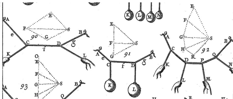
**Figure 5.3.** Reciprocal force diagrams (dotted), from Varignon's posthumous *Nouvelle mécanique, ou statique, dont le projet fut donné en MDCLXXXVII* [New mechanics, or statics, whose project was given in 1687] (See Image Credits at the end of the book.)
