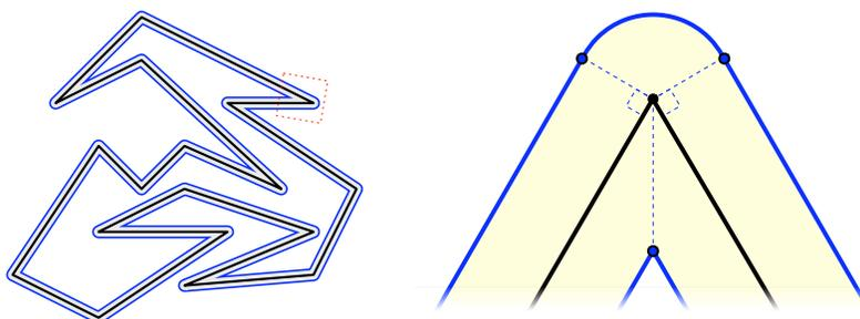
An offset curve  $P_\varepsilon$  and its structure near of a vertex of  $P$ .
